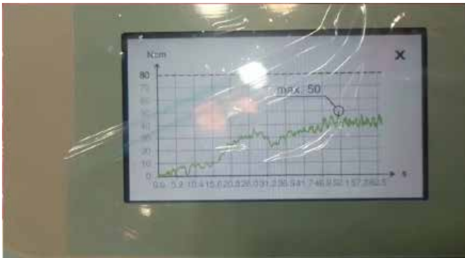
Picture 1- 2: Torque control. W&H Implantmed® device allows monitoring the exact insertion torque during implant placement.
